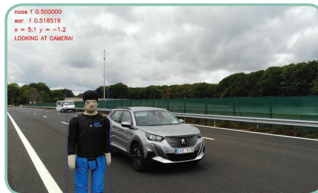
FIG 4 The detection of a dummy face using computer vision.
