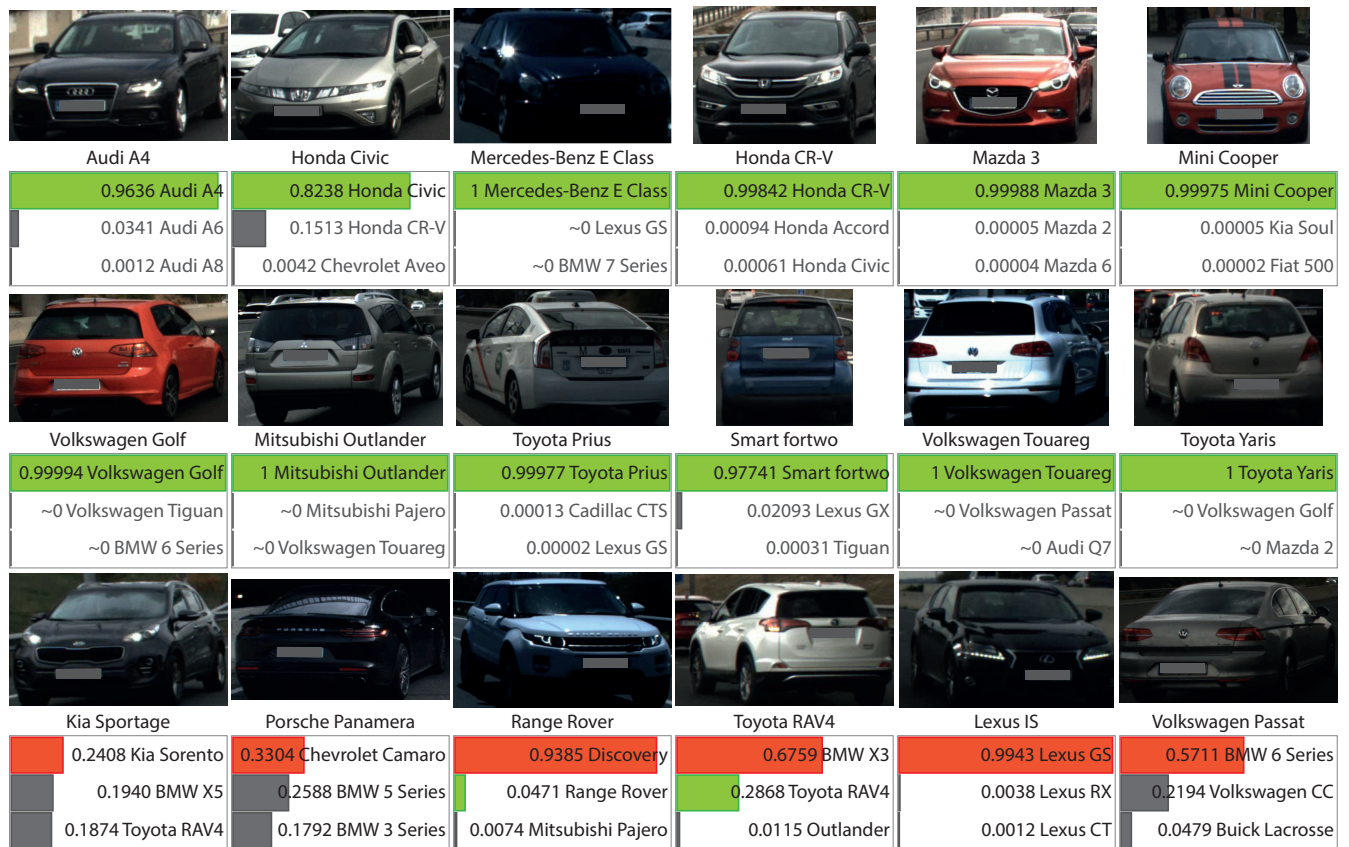
FIGURE 13. Top3 predicted classes of InceptionV3 Fusion-Models model for sample images from the PREVENTION Models test set. The first row shows correctly classified front view images. The middle row shows correctly classified rear view images. The bottom row shows misclassified images from both views.
