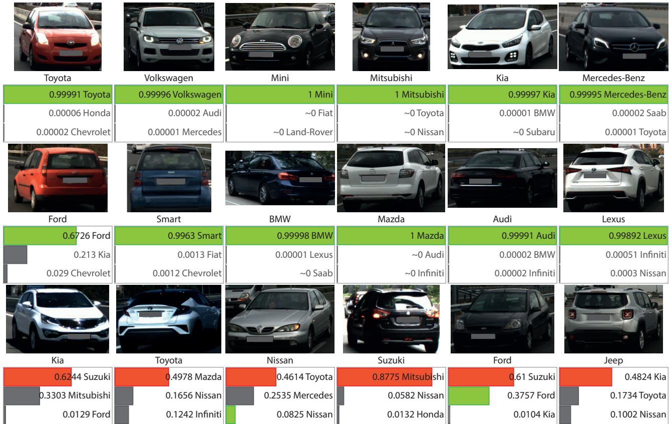
FIGURE 12. Top3 predicted classes of InceptionV3 Fusion-Makers model for sample images from the PREVENTION Makers test set. The first row shows correctly classified front view images. The middle row shows correctly classified rear view images. The bottom row shows misclassified images from both views.
