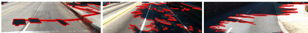
Figure 11. Examples of the results of the shadow edge detection method (images obtained from [19]).
