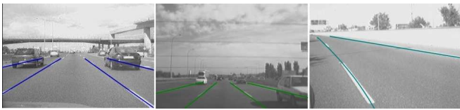
Fig. 4. Vehicle searching area as a result of the lane markings analysis for forward, rear and side modules.
