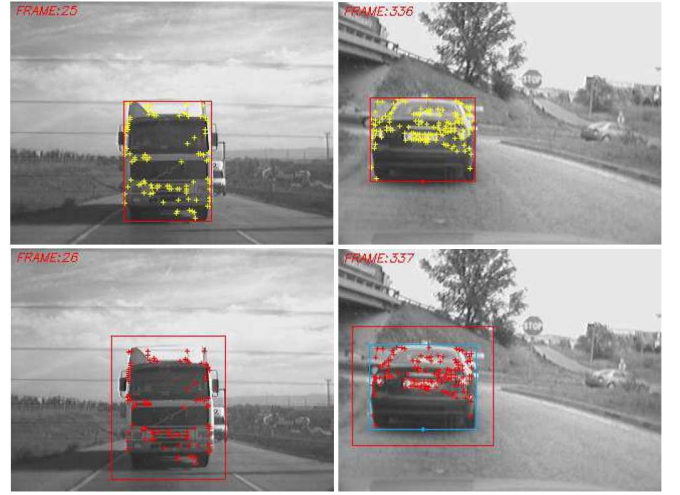
Fig. 10. Data association by features matching. Upper row: Harris features on image t . Lower row: matched Harris features on image t + 1 .
