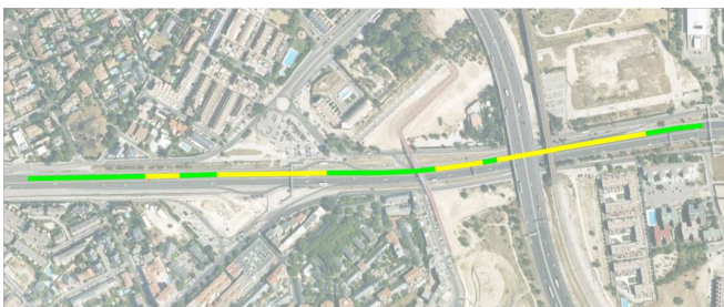
Fig. 17. GPS trajectory and the corresponding traffic load computed at the central unit (the aerial image has been obtained from Google Earth).
