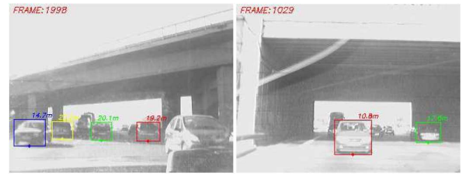
Fig. 12. Examples with strong illumination changes after passing beneath a bridge.
