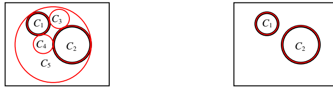
Fig. 3. Circumferences detected using Hough transform for circumferences, applied to the whole image (left) applied to each contour, one by one (right)
