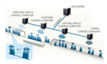
Fig. 11. Control and communication system proposed for OPTIMOTUS.
