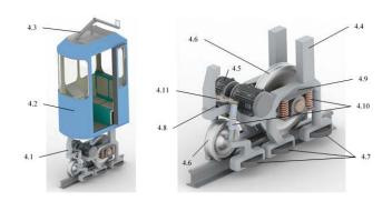
Fig. 4. Preliminary design of a single vehicle of OPTIMOTUS system. Up-isometric compete view, down-rolling stock.
