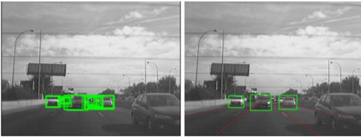
Fig. 4. Left: overlapped candidates. Right: non-maximum suppression results.
