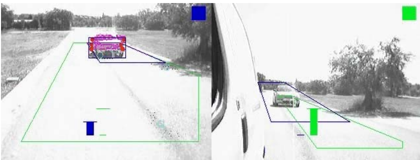
Fig. 8. Panoramic Blind Spot Detection system (Panoramic BSD)
