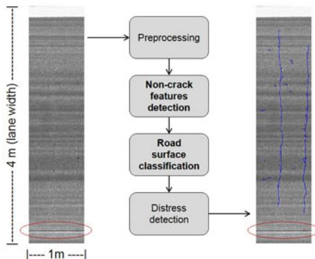
**Fig. 1.** Distress detection system. A global overview.
