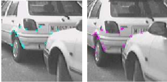
(c) Left image at time 2. Harris points matched with Harris points from Left image at time 1. Outliers from Left image at time 2. in orange
