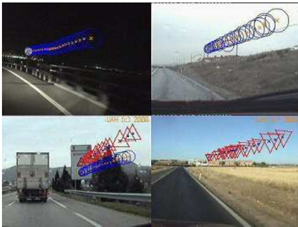
Fig. 6. Traffic sign tracking under different lighting conditions using the Kalman filter. From left to right and up to down: end of forbidden overtaking at night. Same signal with rain drops on the car windscreen. Left bend warning sign and speed limit sign in a cloudy day. Give-way sign in a sunny day.
