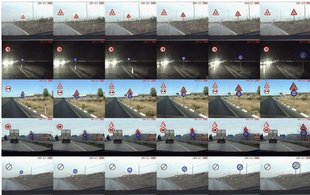
Fig. 8. Sequence of real road images under different weather and light conditions, where circular and triangular signs are detected.
