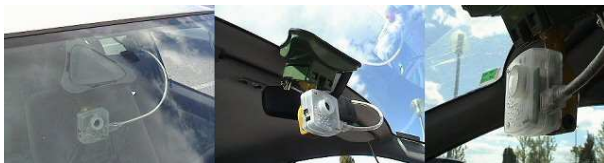
Fig. 7. One camera mounted on the windscreen of the car.
