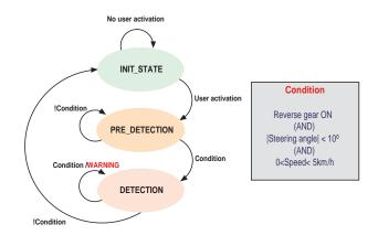
Fig. 4. FSM for detection module.
