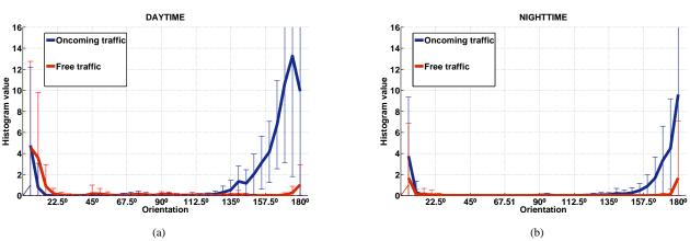
Fig. 9. Mean value of the multivariate Gaussian and standard deviations (square root of the diagonal elements of the covariance matrix) corresponding to both oncoming traffic (blue) and free traffic (red) for (a) daytime and (b) nighttime scenarios.
