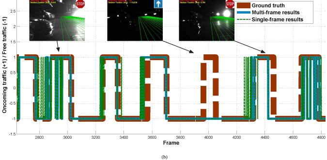
Fig. 12. Examples of nighttime global performance on the test data set. Label "+1" is assigned to oncoming traffic state and label "-1" to free traffic state. Both single-frame and multi-frame system outputs are compared with the ground truth.
