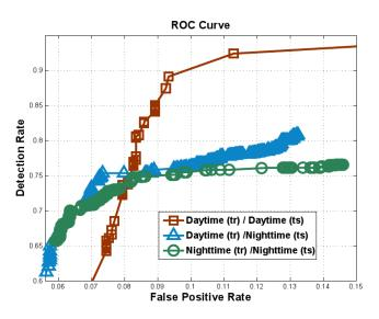
Fig. 10. Receiver-Operating-Characteristic curves of the single frame Bayesian classifiers. We show both daytime and nighttime results, and the results of the classifier trained with the daytime training data set and tested with the nighttime test data set.
