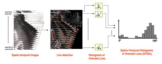
Fig. 7. Overview of the STHOL feature selection architecture.
