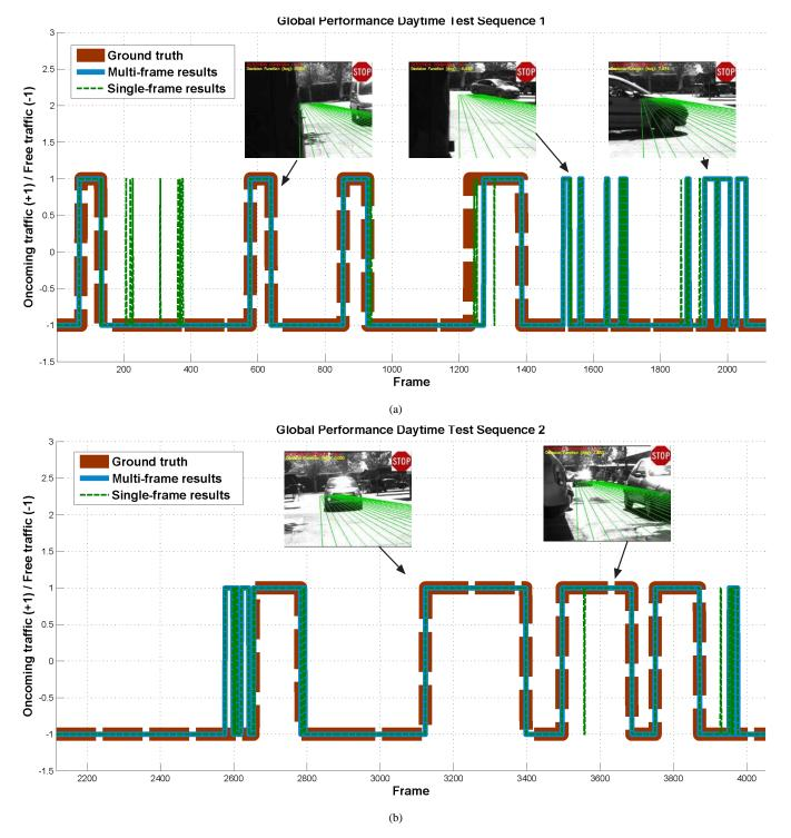
Fig. 11. Examples of daytime global performance on the test data set. Label "+1" is assigned to oncoming traffic state and label "-1" to free traffic state. Both single-frame and multi-frame system outputs are compared with the ground truth.
