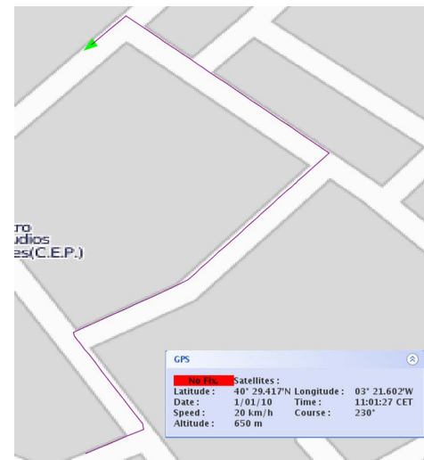
Fig. 9. Vehicle motion trajectory in the OSM and GPS information as shown to the user for the urban canyon experiment.
