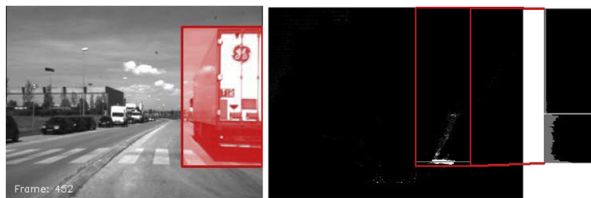
Fig. 6. From left to right: ROI in the original image; XOZ map and the ROI used to compute the length; row histogram and lower bound of the dark area.
