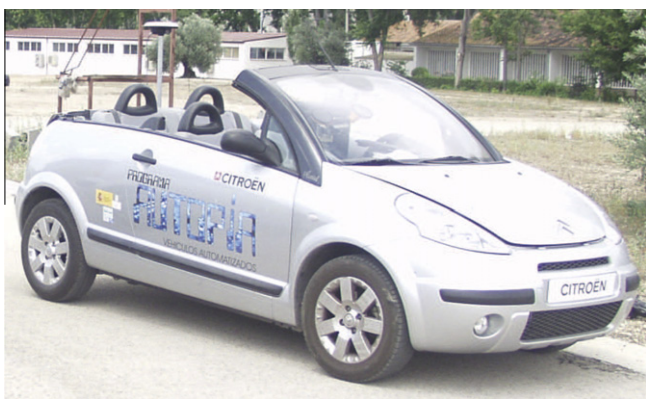
Fig. 2. Automated prototype vehicle equipped with DGPS, IMU, and vision system.
