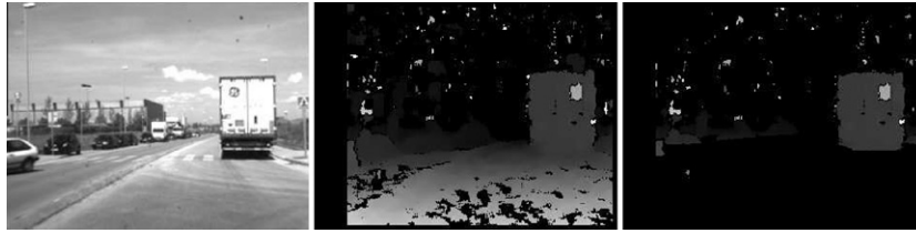
Fig. 4. From left to right: original image, dense disparity map, and filtered map (without ground-plane points or points that are very high).
