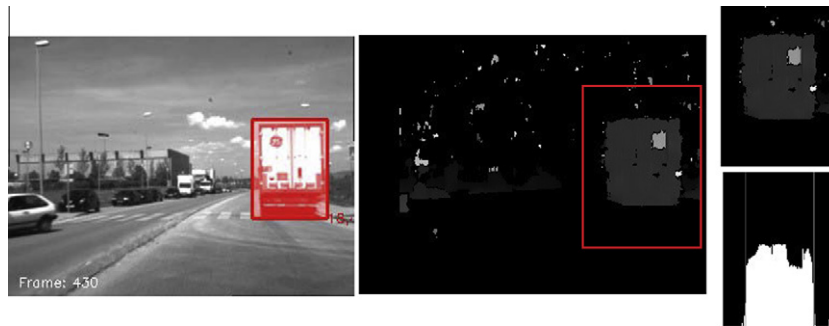
Fig. 5. From left to right: ROI in the original image; enlarged ROI in the filtered dense disparity map; column histogram and lateral boundaries.
